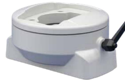
ARM080.830 Rotatable Panel Adaptor Vertical is the connector between the operator panel and the operator arm. The dimension of the adaptor surface is 118x65mm which allows a 315° smooth rotation to the left and right. This product is designed for medium loads and a suitable depth ratio.
