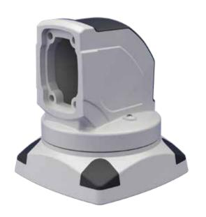
ARM050.600 Rotatable Top Mounted 90° Angle Joint is produced to provide a connection for a high position point. It allows a smooth rotation for the panel horizontally and provides a 315° movement mobility to the right or left. This product is manufactured for light weight configurations.
