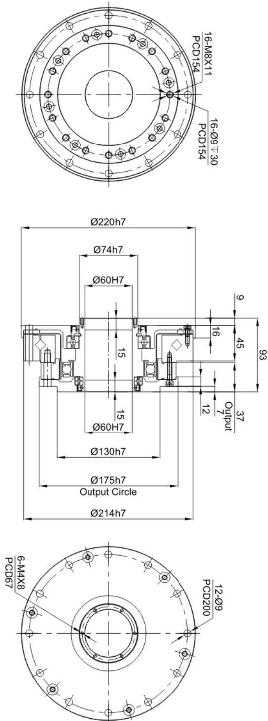
Strain Wave Gear KB-HO Series Box Unit
