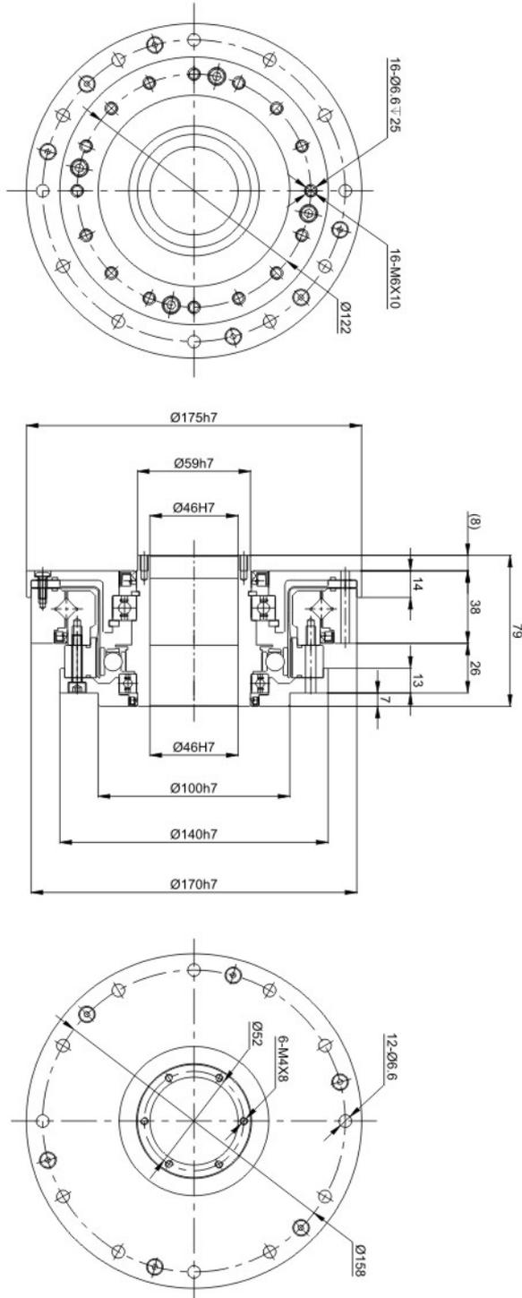
Strain Wave Gear KB-HO Series Box Unit
